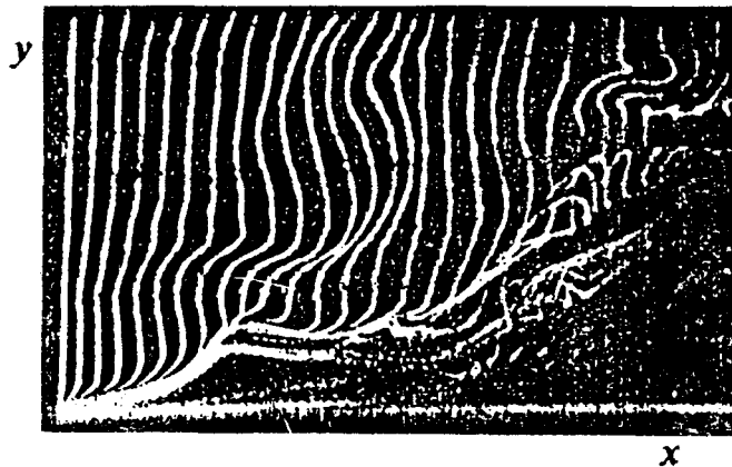
Figure 6. Visualization of a bursting event with the aid of hydrogen bubbles from a pulsed wire (from Kim et al. 7 )
